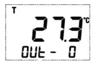
Pressing the LEFT ARROW key selects the location to recall and display. Allow 1 second for data retrieval.
